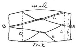
A barrel is used to illustrate the drawing and the hitch. A is the ring; B, hook; C, dotted line, loop under the pack saddle; D, dotted line, loop around the other end of pack saddle; E is the loose end of lash rope, which goes under the saddle (dotted line) F, thus: . . . ; G, loose end as it comes up and goes to the hook, where it is tied.
